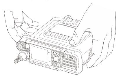
2. Hold the front panel, and then pull and remove the plastic upper cover.
