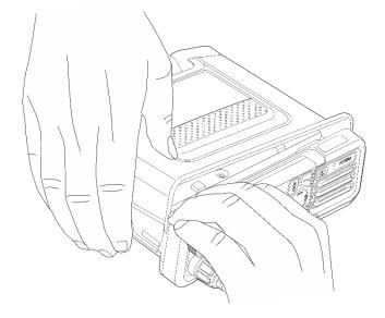
3. Insert the TF card to the metal card slot properly as directed in the following figure.
